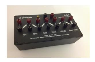
The RS1 is a cost efficient resistance Standard, intended e.g. for use in laboratory, research, metrology and educational applications where a precise yet economical resistance Standard is needed.
